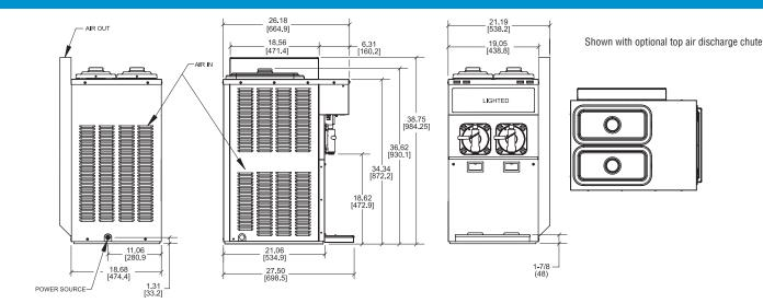
NOTE: FIGURES IN PARENTHESES INDICATE MILLIMETERS. / ALL DIMENSIONS PLUS OR MINUS 1/16 inch [1.5mm].
